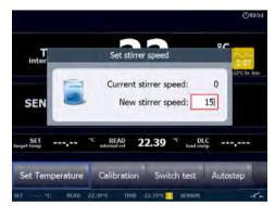
Use the NUMERIC keys to enter a value, or or to accept the value. When pressing the ACTION key or the ENTER key the calibrator returns to the main menu screen.
