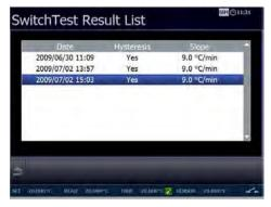
Scroll through the list using the ARROW UP key ▲ and the ARROW DOWN key ▼ and just press ○ or ← to display the result of the highlighted dataset.
