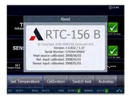
This informs you about the calibrator type, the software version installed, the serial number, the date when it was last calibrated, the build date and the build description.
