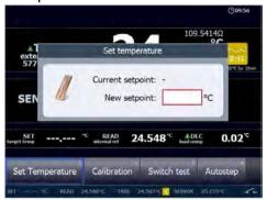
Use the NUMERIC keys to enter a new value, or ○ or ← to accept the value. When pressing the ACTION key or the ENTER key the calibrator returns to the main menu screen.
