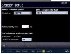
The internal reference sensor will be displayed as the TRUE value on the main screen.
