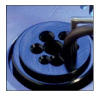
Two special multi-hole insert kits have been developed to comply with the calibration of almost any sensor diameter without having to buy numerous inserts.
