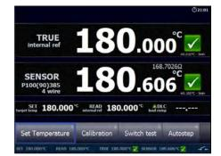
Model B of the RTC is equipped with a built-in accurate measuring circuit for sensor-under-test (input), which enables measurement of virtually any type of temperature sensors including: Resistance thermometers (RTD), thermocouples (TC), transmitters, milliamps (mA), voltage (V) and thermostats.
