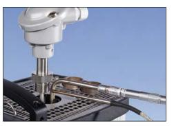
The new STS-200 reference sensors and the DLC sensors have been specially designed. They are both angled 90° and have been customized to fit the calibrator so that they are only slightly higher than the top of the RTC calibrator.
