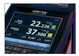
The navigation is menu-driven and very logical to use, and the display shows any important information needed for the current function in use. The communication windows pop up and are followed by discrete sound messages. The display is very bright, and the main information can easily be read from a distance. The avanced simplicity RTC user interface is available in English, German, Chinese, and Japanese.
