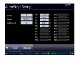
Up to 20 different temperature steps may be programmed including the hold time for each step. Upon completion of an auto-step routine, the user can easily read the results for the sensor-under-test on the RTC display. Results from twenty auto-step calibrations are stored.
