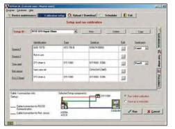
JofraCal is a highly versatile calibration software that is supplied together with the RTC calibrators. The software ensures easy calibration of all kinds of temperature sensors, such as RTD's, thermocouples, transmitters, and thermoswithes. Furthermore, it can be used for pressure calibration i.e. pressure gauges and pressure switches. JofraCal integrates with Jofra calibration instruments. As for temperature calibrators, it is the whole range of temperature
