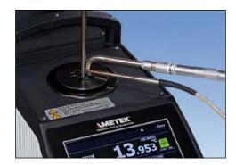
The STS-200 reference sensors and the DLC sensors have been specially designed. They are both angled 90° and have been customized to fit the calibrator so that they are only slightly higher than the top of the RTC calibrator.
