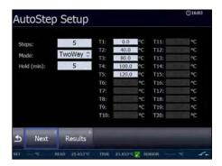
Up to 20 different temperature steps may be programmed including the hold time for each step.
