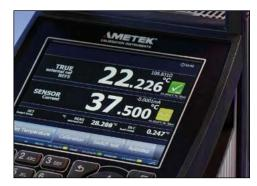
The 5.7" full color VGA display is very easy to read. The main temperatures, like SET, READ, TRUE, and SUT (Sensor under test), are always displayed at all stages of the programming or calibration procedure.
