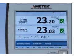
The 5.7" full color VGA display is very easy to read. The main temperatures, like SET, READ, TRUE and SUT (Sensor under test), are always displayed at all stages of the programming or calibration procedure.
