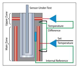
The PTC series of calibrators provide precision temperature calibration of sensors, whatever the type or format. This is accomplished through an innovative active dual-zone heating technology.
