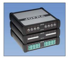
Using the JOFRA PTC series together with the ASM, Advanced Signal Multi-scanner, offers a great timesaving automatic solution to calibrate multiple temperature sensors at the same time. The ASM series is an eight channel scanner controlled by the JofraCal software on a PC. Up to three ASM units can be stacked to calibrate up to 24 sensors at a time. It can handle signals from 2-, 3- and 4- wire RTD's, thermocouples, transmitters, temperature switches, and voltage.
