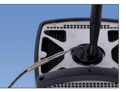
The STS-150 reference sensor is specially designed with an angled 90° rod, and customized to fit the calibrator so that it is only slightly higher than the top of the PTC calibrator. The unique design makes it possible to calibrate threaded sensors and sensors with connection heads without any problems. The STS-150 reference sensor also alerts you when your calibration has expired.
