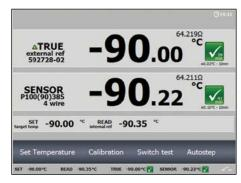
Model B of the PTC is equipped with a built-in accurate measuring circuit for sensor-under-test (input), which enables measurement of virtually any type of temperature sensors including: Resistance thermometers (RTD), thermocouples (TC), transmitters, milliamps (mA), and thermostats.
